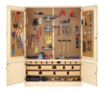
**Diversified Woodcrafts** Cabinet is constructed of solid maple and maple veneers. Upper cabinet doors, side and rear panels are lined with 1/4" pegboard. Lower cabinet features 1 fixed and 2 adjustable 1" plywood shelves. Upper and lower locking doors of 1-1/8"T maple veneer panels mounted with hinges. Earth-friendly UV finish. Shipped set up.
